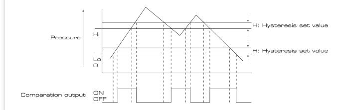
When the pressure large than value (Hi) or less than value (Lo), the output is OFF. When pressure large than value (Lo) and less than value (Hi), the output is ON.
