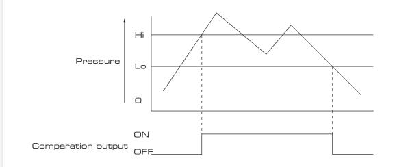
When the pressure is large than (Hi) value, the output is ON. When the pressure is less than the (Lo) value, the output is OFF
