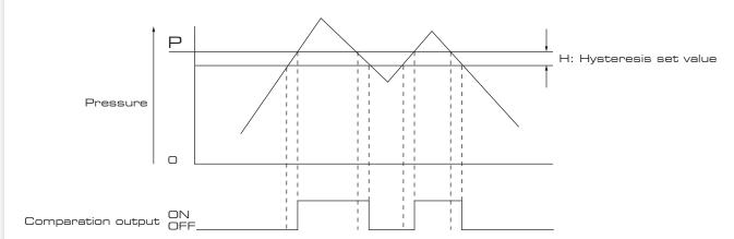
When the pressure is large than (P) value, the output is ON. When the pressure is less than the (P) value, the output is OFF
